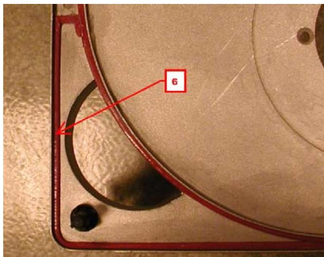
5. Addition of a seal groove, removed the gasket and now use only of one type of cam (standard cam for streamline - not shown here, only delivered as spare parts for the forced flue burners)
