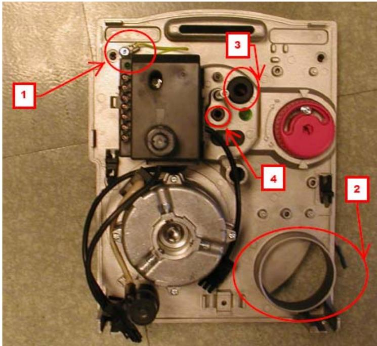
1. New fastening of the earthing pin (anti-rotation of the pin)
