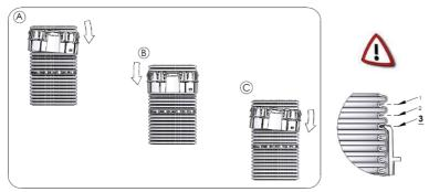
e) Fit the gasket 5 in the first groove of the flexible pipe,
